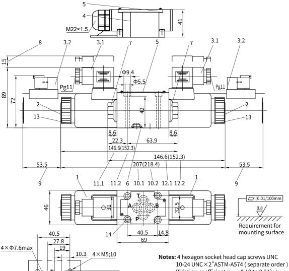
(Friction coefficient  $\mu_{total}$ =0.19 to 0.24); Tightening torque  $M_A=11Nm$  [8.2ft-lbs]  $\pm 15\%$ 31 75 (Friction coefficient  $\mu_{total}$ =0.12 to 0.17); Tightening torque M<sub>A</sub>=8Nm [5.9ft-lbs] ±10%
